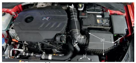
6. Remove the fastener [4] in the middle in front of the battery
