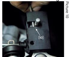
14. Insert Allen screw [11] and tighten it with 11 Nm
