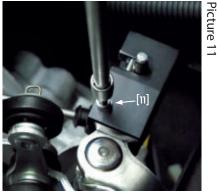
15. Check that the short shifter is fixed firmly in place16. Check again that the gearshift is functioning correctly
