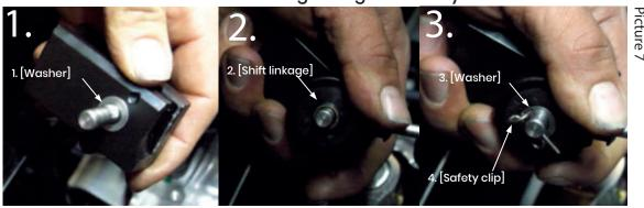
12. Carefully slide short shifter onto shift cable mount
