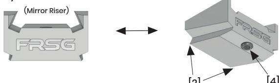
1. Carefully unclip the cover in the direction of travel (CAUTION: DANGER OF BREACH!)
